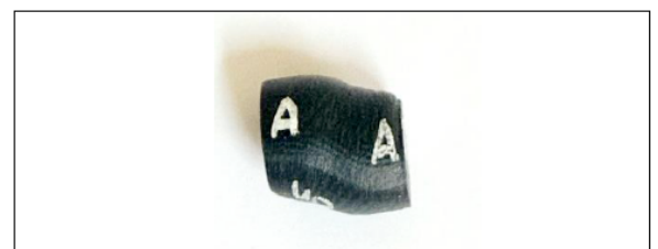
Figure 4: Buckling occurred in the compression test sample of 25.4 mm length.
