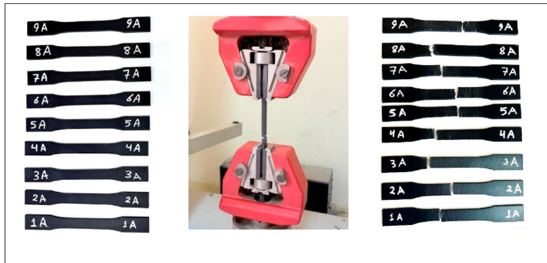
Figure 3: Tensile strength specimens of Hyper PLA-CF prior to, during, and following testing conducted with the Universal Testing Machine.
