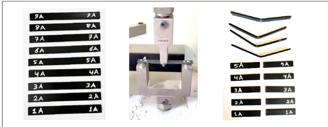
Figure 6: The bending strength specimens of Hyper PLA-CF before, during, and after testing, as measured by a universal testing machine.
