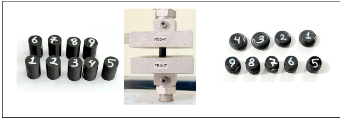
Figure 5: The compression strength samples of Hyper -PLA-CF depicted before, during, and after testing, with the utilization of a universal testing machine.
