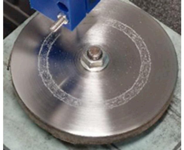
Figure 9: Formation of thin PLA film on the contact surface.
